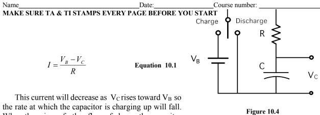
the rate at which the capacitor is charging up will fall. When there is no further flow of charge the capacitor will be fully charged to its final value,
