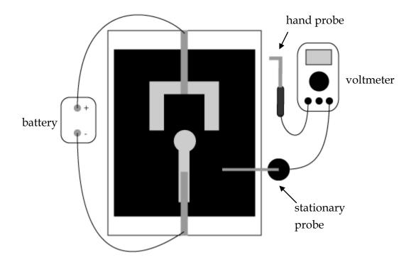
Figure 7.4. Field Mapping Apparatus
